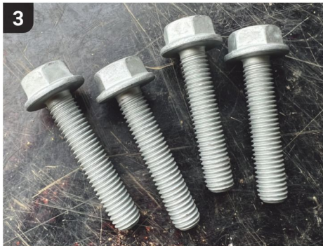
Each mount requires two new 13mm bolts. Don't reuse the old bolts. Available from Design 911's online store (alongside the Rohler mounts), the new bolts can be found under part number 90037805501.
