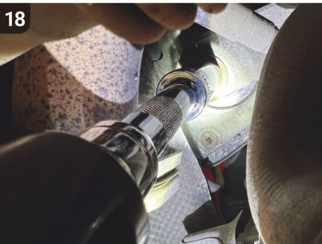
18 This is the view from underneath the engine mount. Take an 18mm deep socket on the end of a ratchet extension and breaker bar, crack the old mount's bottom nut free, then unscrew and remove it.
