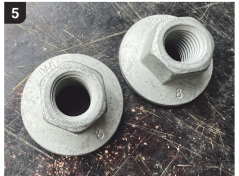
If you've decided to replace tired factory mounts with new OEM parts (if so, expect to be doing this job again in the near future), you'll need new 18mm retaining nuts, part number 99908421501.
