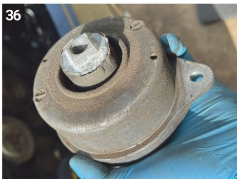
36 Unfasten the old engine mount bolts and discard them. Pull the old engine mount free.
