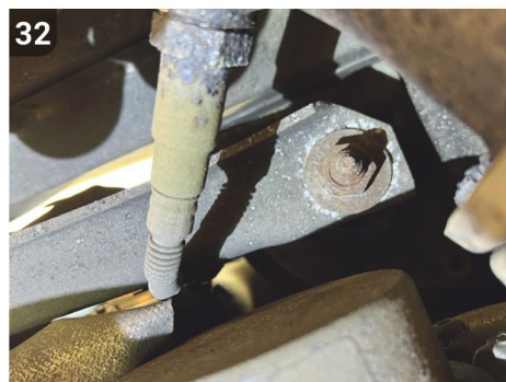
32 Here is the offside engine mount lower nut, seen from beneath the car. This area is more heavily populated with parts than where you were working on the nearside. A flashlight will prove useful.
