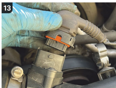
You will now need to remove the mass airflow sensor connector plug located atop the air box. Press the clip on the engine-side half of the plug and wiggle it free.
