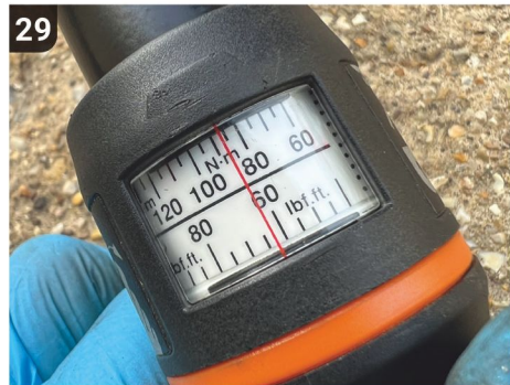
29 The bottom bolts need to be tightened to the manufacturer's recommended torque setting of 63lb-ft. Again, use your torque wrench to ensure the correct value is applied.
