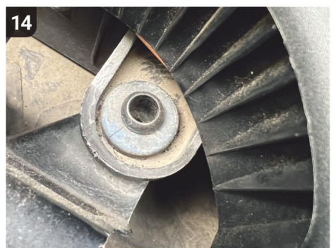
Unclip the mass airflow sensor plug wiring from the back of the air box, which is held in place by locating lugs fed into rubber grommets. No tools are needed for removal. Pull the air box free of the engine bay.
