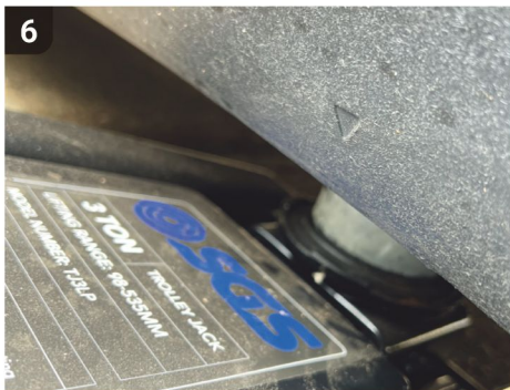
Lift the Porsche a few inches off the ground in order for you to be able to use a ratchet extension to reach each mount's bottom bolt. Use axle stands to support the vehicle securely.
