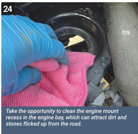
Pictured is the engine mount locating hole. This matches the shape of the locating notch on the base of the new engine mount.
