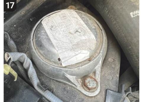
17 We'll replace the passenger-side engine mount first. Engine mounts should be replaced in pairs, but we suspect this mount was installed on its own and more recently than the offside engine mount.
