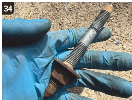
34 Take your 18mm deep socket and crack the nut free, then unscrew it. As you can see, this entire bolt assembly has become separated from the engine mount body. This won't have helped handling!
