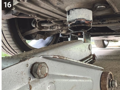
16 Move your jack (or use a second jack) to support the weight of the engine, which you may need to lift a few millimetres, depending on how much the old mounts are sagging. Use a rubber jack pad.
