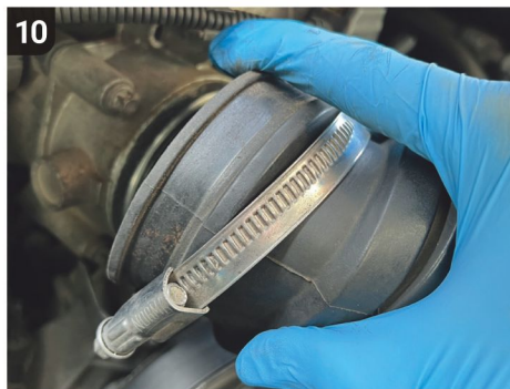
With the jubilee clip undone, carefully pull the rubber intake hose away from the throttle body.
