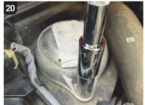
20 Back in the engine bay, use a 13mm socket to unscrew the old engine mount bolts. If they have been overtightened, use your breaker bar to crack them off before unscrewing.
