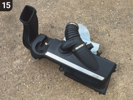
15 Put the air box assembly to one side. You will now have uninhibited access to the engine mounts. This is a good time to replace your Porsche's air filter, should you suspect the part is past its best.
