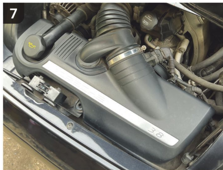
You will also need to remove the air box for ease of access. It should be noted, Rohler mounts won't adversely affect ride quality or trigger knock sensor warnings (commonly associated with solid mounts).
