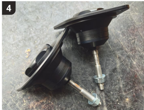
Design 911 supplies Rohler semi-solid engine mounts in pairs, complete with the required 19mm nuts and washers, though you'll need to order the aforementioned 13mm bolts.
