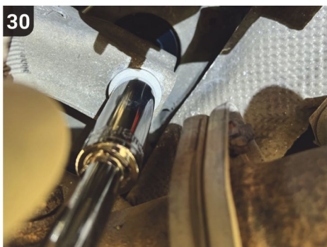
30 Back underneath the car, take a 19mm deep socket on the end of a ratchet extension and tighten the new Rohler engine mount lower nut. Make sure you've included the new washer.
