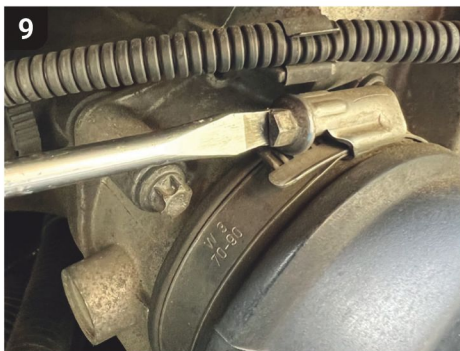
Next, take a flat-headed screwdriver and use it to loosen the jubilee clip fastening the air box intake hose to the throttle body assembly.
