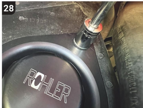
28 Using a torque wrench, tighten the 13mm bolts to the manufacturer's recommended torque setting of 23lb-ft. Our old mount's bolts were hugely over-tightened. Don't make the same mistake!
