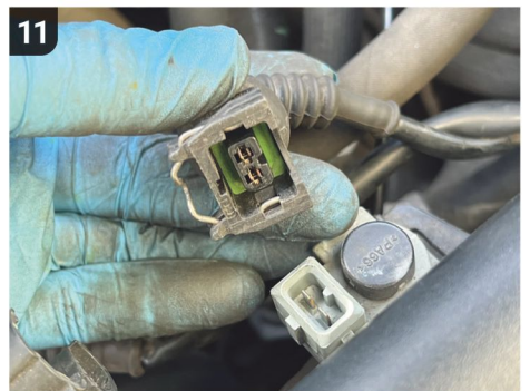
A vacuum solenoid is attached to the rear of the air box. You can leave the solenoid in place, but unplug it from the wiring loom.
