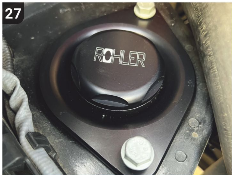
27 With the Rohler engine mount placed in its new home, put your new 13mm fastening bolts in place and finger-tighten them, ensuring the mount is sitting comfortably.
