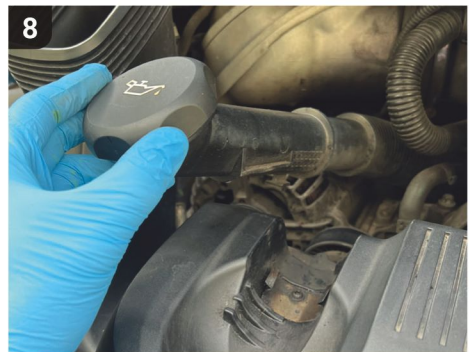
Our car is a first-gen 997, but the following steps are virtually identical for the 996 and second-gen 997. The Rohler mounts suit all models. Begin by pulling the oil filler neck away from the air box.
