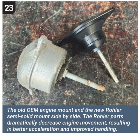
You should now be able to pull the old engine mount free from the engine bay. The rubber visible here appears compressed, suggesting the mount is well past its useful service life.
